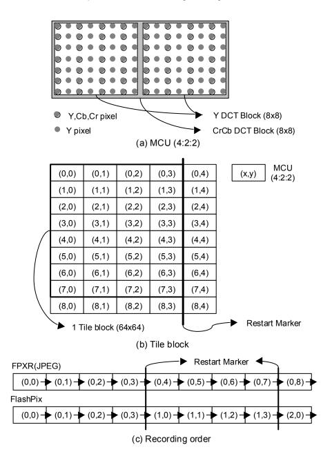
Figure 59 Conversion to Flashpix Using Restart Markers
