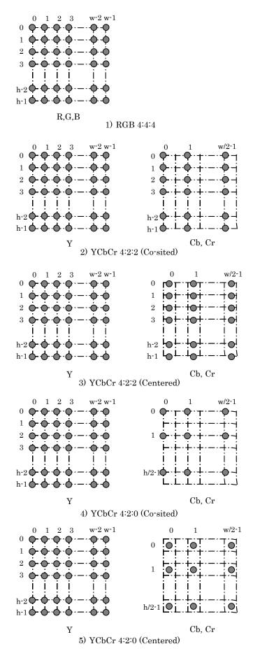
Figure 4 Pixel Composition and Pixel Sampling
