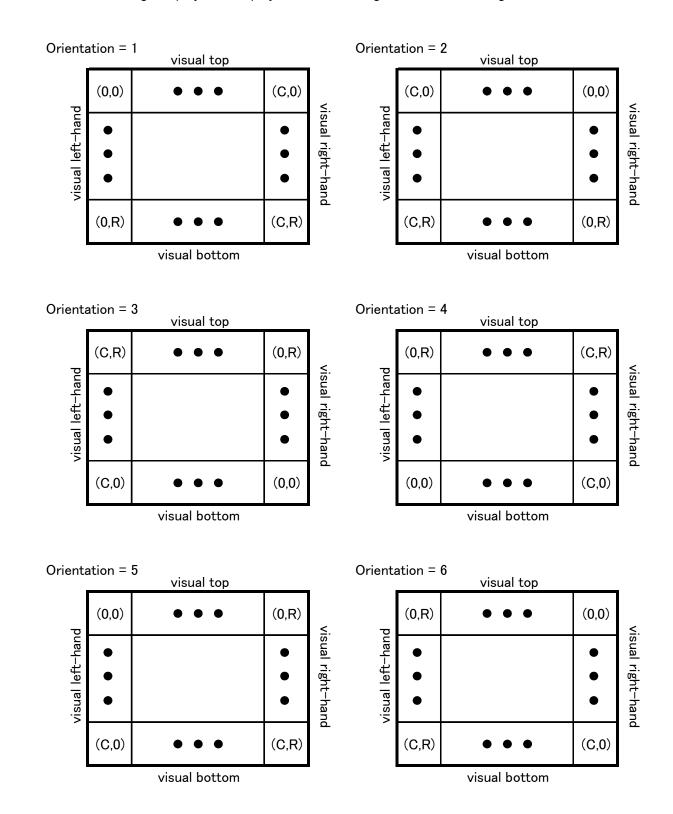
**Figure 12** shows the relationship between coded image data that is stored in an Exif image file and orientation of the image display on a display screen according to the orientation tag.
