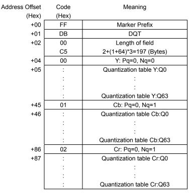
Figure 24 DQT Structure (with three quantization tables)
