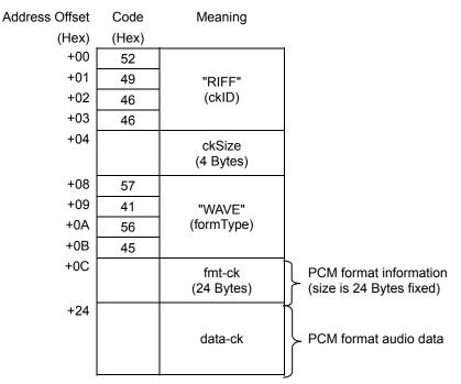
Figure 44 Basic Structure of PCM Format
