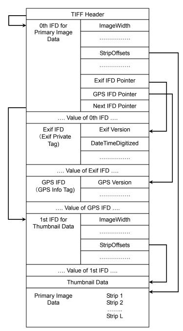
Figure 6 Basic Structure of Uncompressed Data Files
