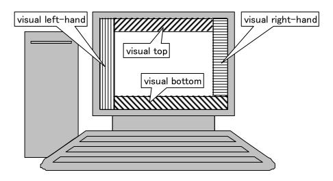
Figure 11 Orientation of an image display on a display device
